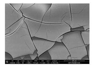
Figure 5: SEM Image of the sample showing flakes
