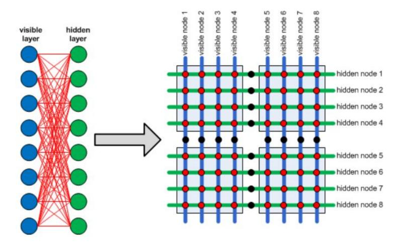
Figure 4 Embedding of RBM visible and hidden nodes onto D-Wave chip layout
